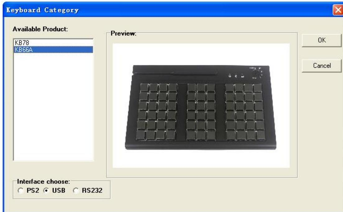
First, selecting the interface; second, selecting the model of the keyboard; and then clicking “OK”.
