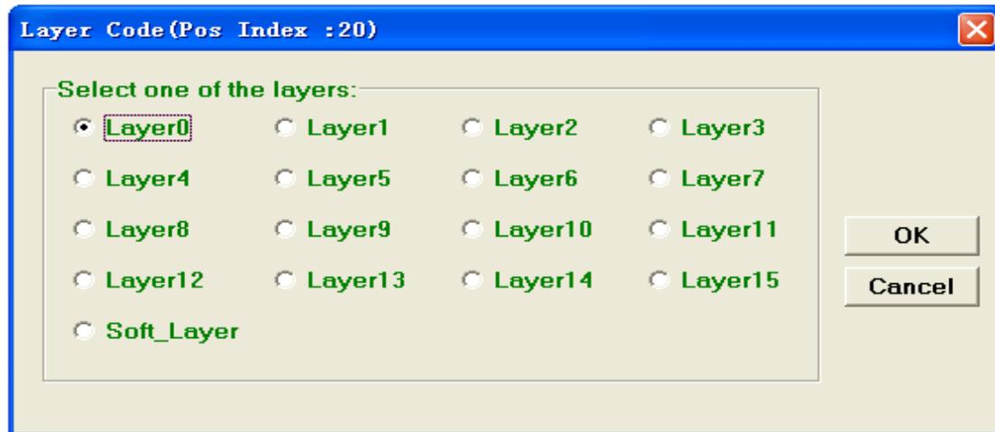
For instance, if you want to define the key cord on the “Layer3”, you can select “Layer3” in the menu and set the key code through scan code mode. After finishing it, you need to set a toggle key of the layer by the layer index. As the following shown:
